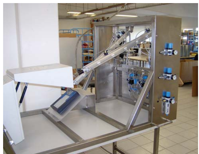
Mechanical life test of the 4921 RF Shield
