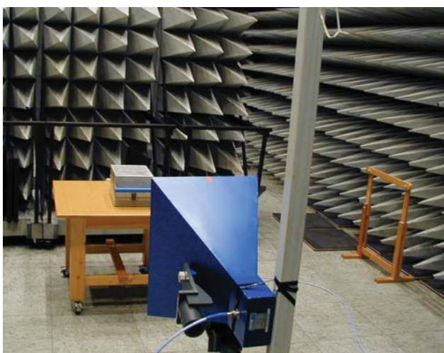
4921 RF Shield with transmitting antenna in EMC laboratory
